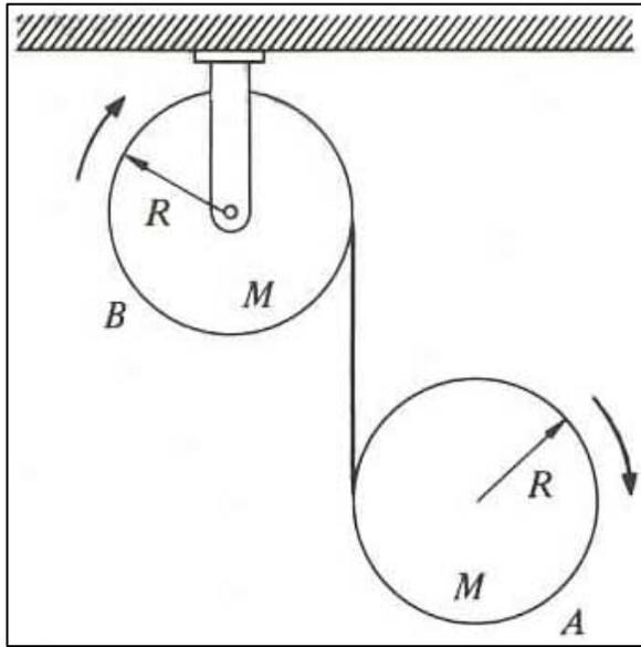
A drum  $A$  of mass  $m$  and radius  $R$  is suspended from a drum  $B$  also of mass  $m$  and radius  $R$ , which is free to rotate about its axis. The suspension is in the form of a massless metal tape wound around the outside of each drum, and free to unwind. Gravity is directed downwards. Both drums are initially at rest. **Find the initial acceleration of drum  $A$** , assuming that it moves straight down.
