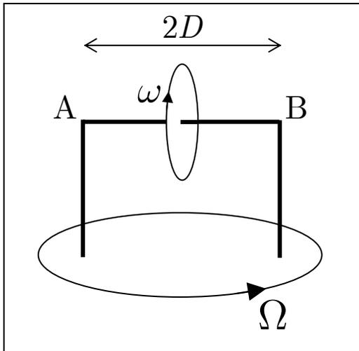
A disc rotates at an angular velocity  $\omega$  and is mounted on a turntable which rotates at a velocity  $\Omega$ , as indicated in the diagram. **Find the magnitude and direction of the forces on the wheel's axle at the points labelled  $A$  and  $B$  in the diagram.**
