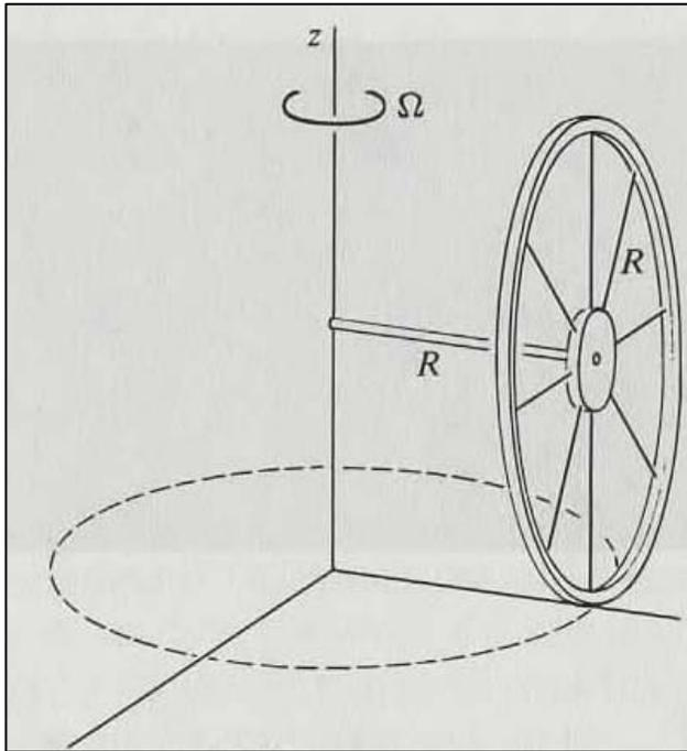
A thin hoop of mass  $m$  and radius  $r$  rolls without slipping about the  $z$ -axis. It is supported by an axle of length  $R$  through its centre. The hoop circles around the  $z$ -axis with angular speed  $\Omega$ . [Note: the moment of inertia of a hoop for an axis about its diameter is  $mR^2/2$ ]
